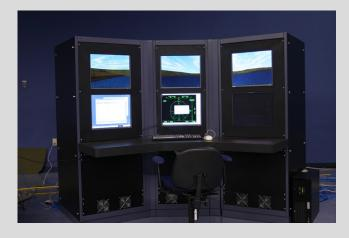
The instructor station software provides complete simulator control with an extensive set of features that include malfunctions, freezes, initial conditions, environmental control, and aircraft repositioning. The instructor station graphical user interface has a modern look and feel and is designed for touch screen use.
